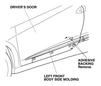
13. Using a rubber roller, apply pressure against the body side molding and roll from one end to the other.
