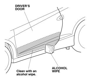
2. Using one alcohol wipe, thoroughly clean the driver's body panel where the left rear body side molding will attach.
