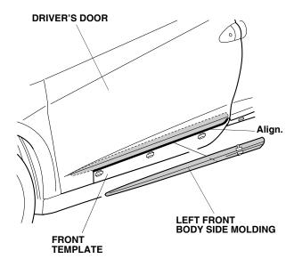
9. Peel back approximately 1½ to 2 inches of adhesive backing from each adhesive strip, and tape the ends to the front surface of the body side molding.
